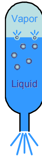
Figure 1: VaPak uses the internal energy of the fluid to pressurize the tank.
