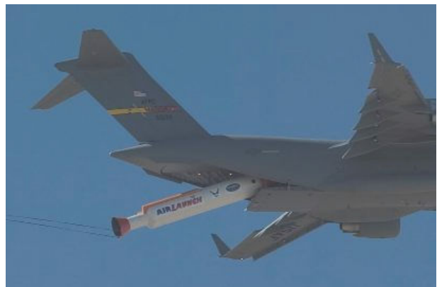
Figure 8: QuickReach VaPak driven Small Launch Vehicle test article deployed from a C-17 airplane. (courtesy of AirLaunch LLC)
